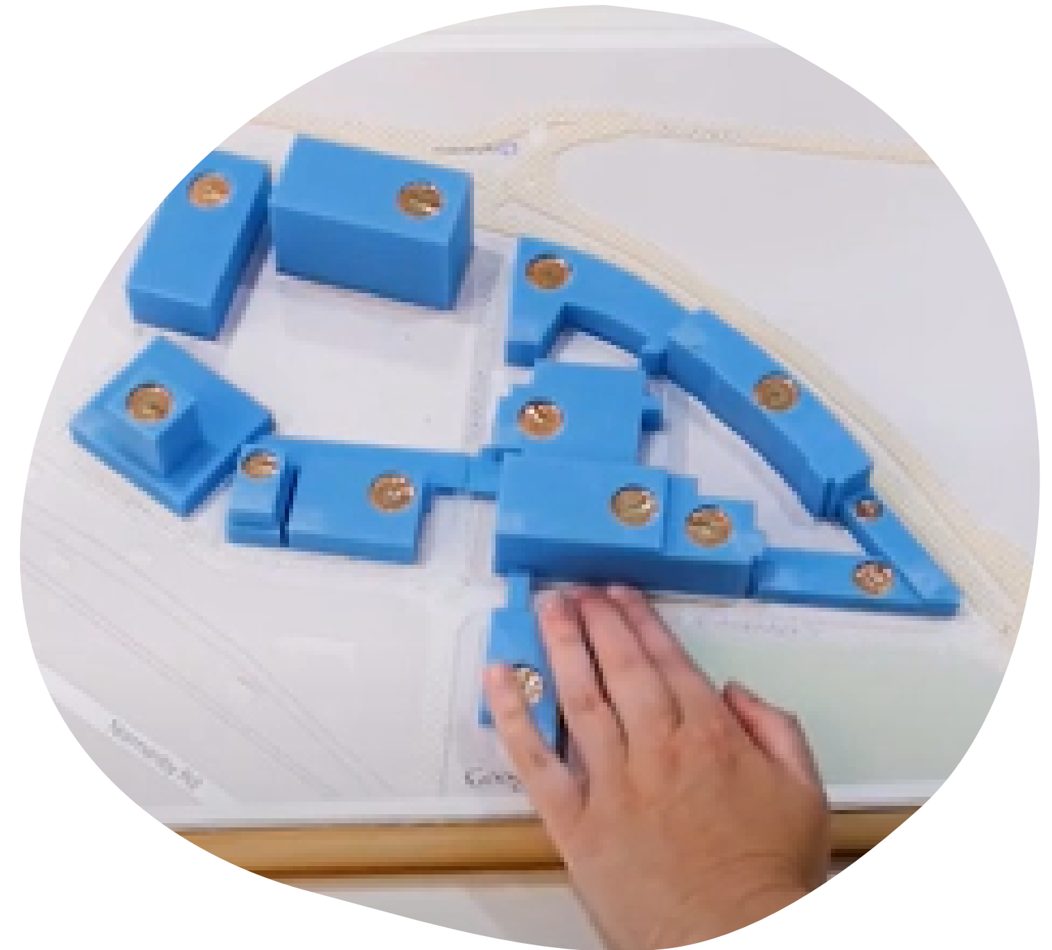
Tactile map made with 3D printer for blind people
