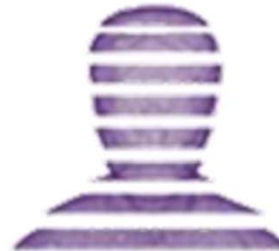
Layer Slices & Tool Path
